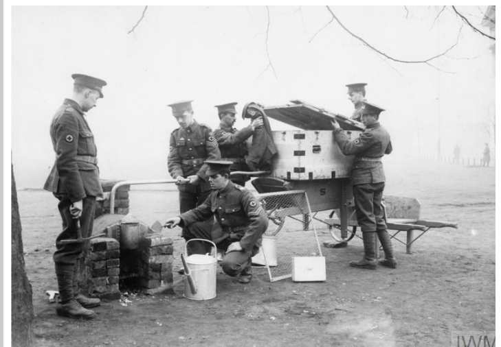
FIG. 1.—PORTABLE STEAM DISINFECTING APPARATUS (THE THRESH'S)
